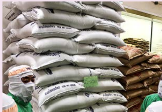
Advice Not to Over-stack Auxiliary Feedstock
