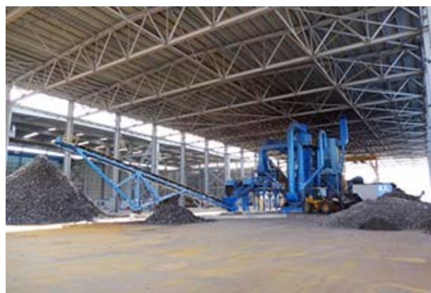
The state-of-the-art ultra-large shredder equipment is made in the United States and boasts 6,000 horsepower
