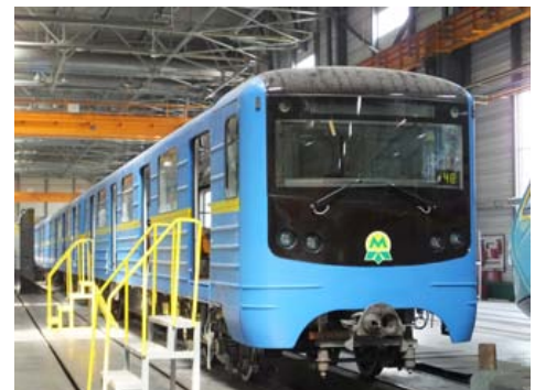
Modernized metro train assembled with Japanese AC propulsion at Kryukovsky Railway Car Building Works
