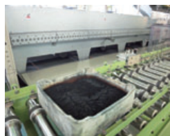
Raw materials are mixed and placed in the container, which is then transferred to the firing machine, which functions like an oven.
