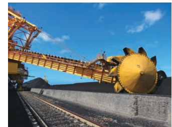
Large reclaimer in operation as coal is loaded onto belt conveyor
