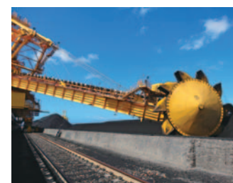
Large reclaimer in operation as coal is loaded onto belt conveyor
