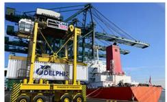
Straddle Carrier with Hydrogen Engine
