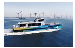
Offshore Wind Support Vessel with Hydrogen Engine
