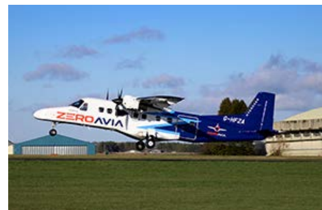
Demonstration flight with ZeroAvia's hydrogen-electric engines installed on a 19 seat Dornier 228 aircraft
