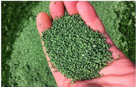
PRO-gran crumb rubber made by casing tyres
