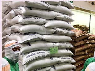
Advice Not to Over-stack Auxiliary Feedstock
