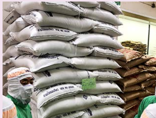
Advice Not to Over-stack Auxiliary Feedstock
