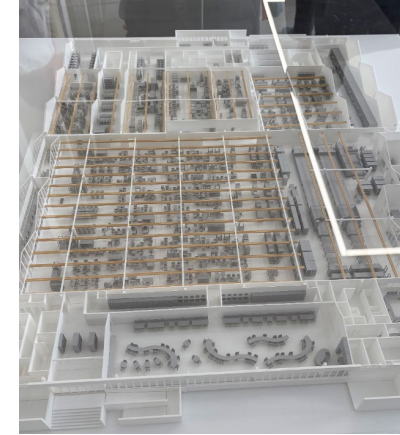
All processes, from raw material arrival to product shipment, are consolidated on a single floor.
