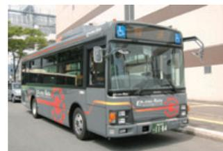
LiB-powered electric bus in operation in Akita Prefecture
