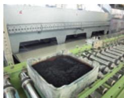
Raw materials are mixed and placed in the container, which is then transferred to the firing machine, which functions like an oven.
