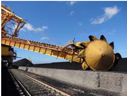
A large reclaimer in operation as coal is loaded onto belt conveyor.
