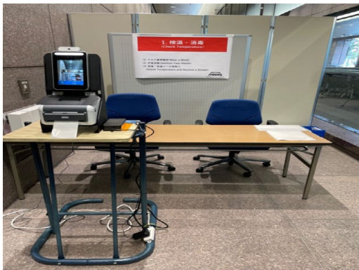
Temperature check station with a machine that takes the patient's temperature and issues a sticker with the temperature printed
